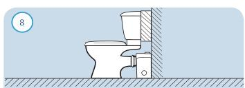
maintenance being required. If boxed in, the boxing should be easily removed. Any extension between the WC pan spigot and wall should not exceed 150mm.
