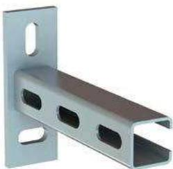
**Usage:** universal channel system for building fastening systems, with repeatable perforation; with cut centimetre scale on the channel side.
