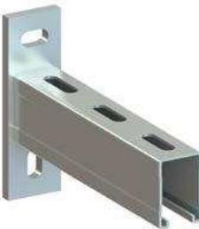
**Usage:** universal channel system for building fastening systems, with repeatable perforation and serrated edges in order to lock the accessories better; with cut centimetre scale on the channel side.
