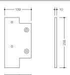
Mounting plate hinged support rail hinged support rail right handed version
