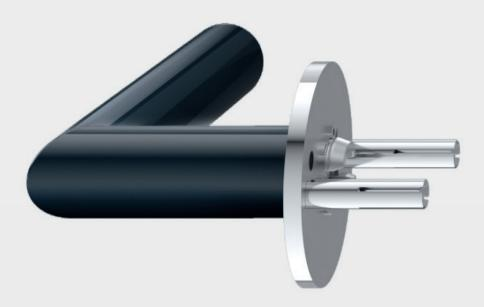
The innovative mounting technology of the flat rose enables extremely fast and permanent fixing without screws For the fixing, latching sleeves and threaded bolts are pushed i to each other, so that they lock together and are pull-resistant. The quick connection makes installation and dismantling simple. Fire door fitting sets to DIN 1827 complete the projects range.
