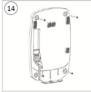
14 Screw the Plug-in base to the wall(x4)
