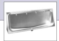
Urinal through in stainless steel, for wall mounting. Two alternative 1/2" connections, one concealed and one visible. Supplied with 1 1/2" grated waste, screws and fixing bracket. Supplied with 4 flushing heads.
